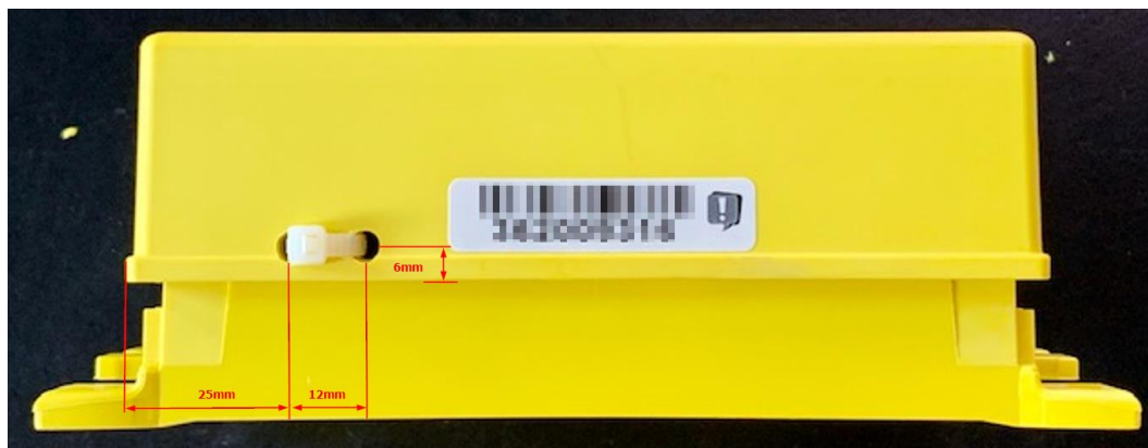
Figure 5: Fall protection with cable tie
