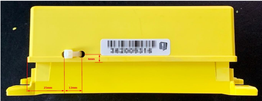
Figure 16: Fall protection with cable tie
